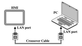
For more details about HMI via Ethernet port on uploading and downloading, refer to [Advanced part 7 Compile /
