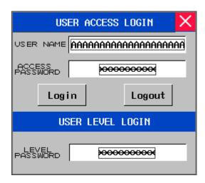
[Frame9: Login Window] is for inputting passwords of security levels and user permissions. User using security level function only need to input appropriate password of security level.
