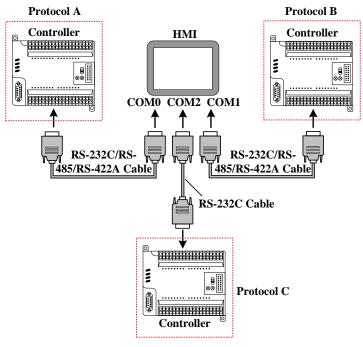
[Example] Below a GH070E with a SIEMENS S7-200 (hereinafter referred to as PLC 0), a MITSUBISHI FX2N (hereinafter referred to as PLC 1), an OMRON CP1H (hereinafter referred to as PLC 2) communication, for example, Requirements were monitored on the HMI PLC 0 of VW 100, PLC 1 of D100 data and PLC 2 in Q 0.0 outputs.
