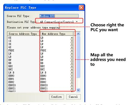
The user can select the replace PLC type in the pull-down list of the destination PLC type, and the user select new address types in address type mapping list according to the address type relationship between source PLC type and destination PLC type.
