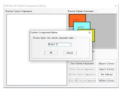
(3) Enter in the custom component name: Figure 1, click [OK], then these 3 rectangles will be added to the newly created custom component library named [Group] with the name [Figure 1]. As shown in the image:
