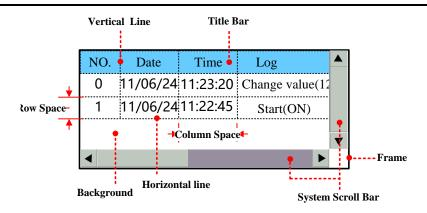
\* When the operation log cannot be wholly displayed in vertical or horizontal direction, system will provide scroll bar automatically. The width of system scroll bar can be set in HMI Extend Attributes of HMI Attributes; the width is optional from 20 to 120(pixel).
