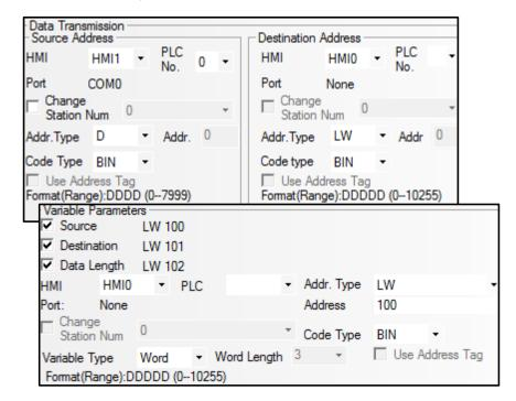
When the offset of Source Address is 0, offset of Destination Address is 0 and the Data Length is 1:
