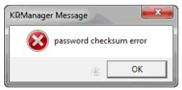
Only enter password correctly then project can be downloaded into HMI.
