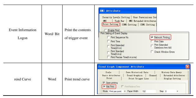
[Example]: requirements through remote printer to print the HMI Screens.
