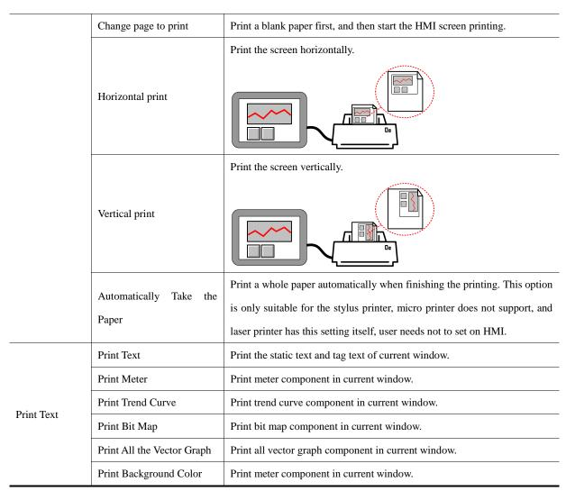
Method 2: Do not check the Custom Print Options; use the bits of LW9054 and LW9055 to set the print.
