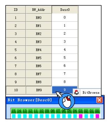
[Examples] For example RW9 value is 9, bit browser form RW9: 03,00 bit address can be seen in red: ON, decimal 9 to binary form as 0000 0000 0000 1001.
