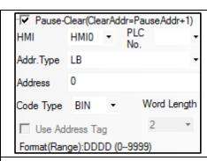
Set the register to turn page of multiple pages of XY Plot, the default word length is 3. This option is valid when the Multiple Pages is chosen. Use this function to scroll the multiple pages XY plot, and can be used
