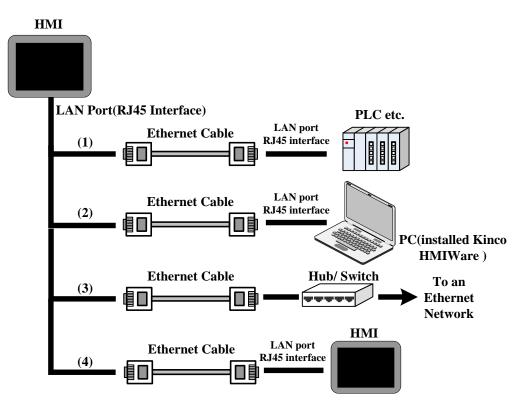
(1) Connect with PLC and such controllers to communicate
