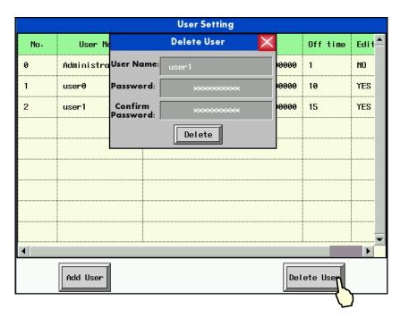
Input the user's name to be deleted and the corresponding password, confirm it, and then click "Delete" to complete the operation.
