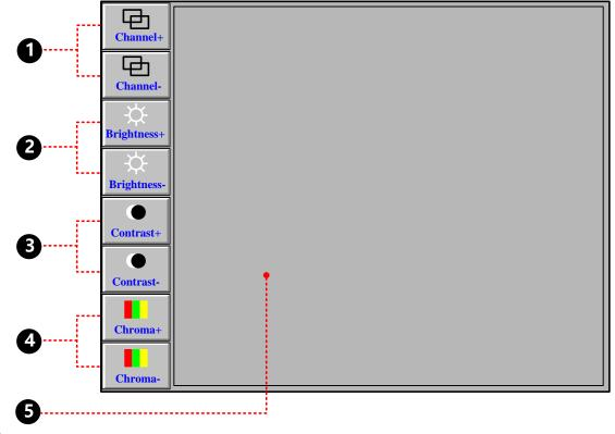
• Multiple State Setting component, it is used to switch the channels (There are only 2 CVBS port on MT5620T), its
