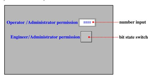
Create a number input component and a bit state switch component, and the attribute setting is as follows:
