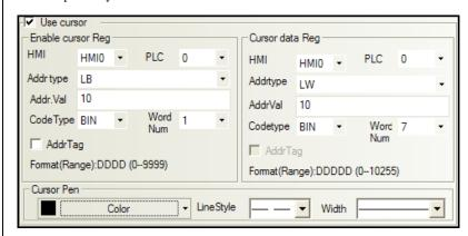
As following picture: Set Enable Scroll AddressLB0 to ON, then Scroll Data Address LW10, LW11, LW12, LW13, LW14, LW15 correspond to second, minute, hour, date, month, and year of the sampled data respectively. LW16 corresponds to data value of channel 0; LW17 corresponds to data value of channel 1, and so on.
