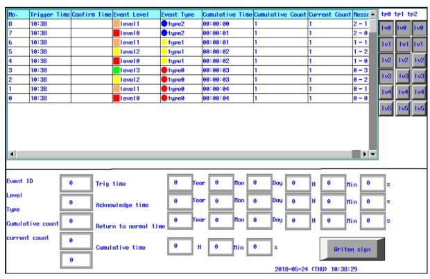
8. Click on one of the alarms (confirm the alarm), and output the alarm to the details:
