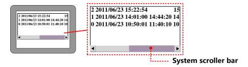
The width of system scroll bar can be set in [HMI Attribute]—[HMI Extended Attributes], the range is 20~120 (Pixel).
