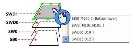
You can use the tool bar (set top/set bottom/ previous layer/next layer) to adjust the layer position of the stacked components
