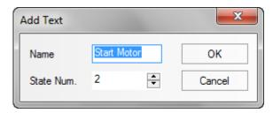
For example, build a text item named "Start Motor", the State Num is 2, each text supports 256 states at most. Click on the Ok to finish building the text, and click on the Cancel to give up this text.
