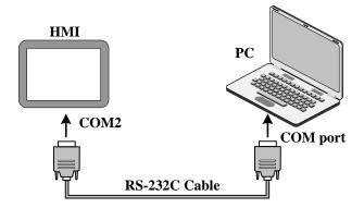
For more details about uploading and downloading via the serial port on the HMI, please refer to [Advanced Part 8]
