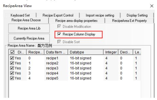
2.The left column shows the list of recipe parameters, and the right column shows the corresponding recipe content.
