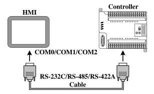
[Example] Below a GH070E with a SIEMENS S7-200 communication, for example, requires the HMI monitor PLC M0.0 output state. (This example uses the HMI COM0 port to connect PLC communication)
