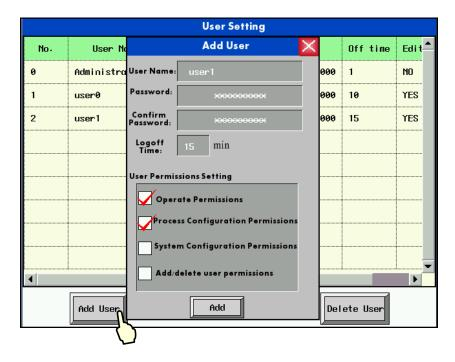
Input the user's name to be added and the corresponding password, confirm it, then click "Add" to complete the operation.
