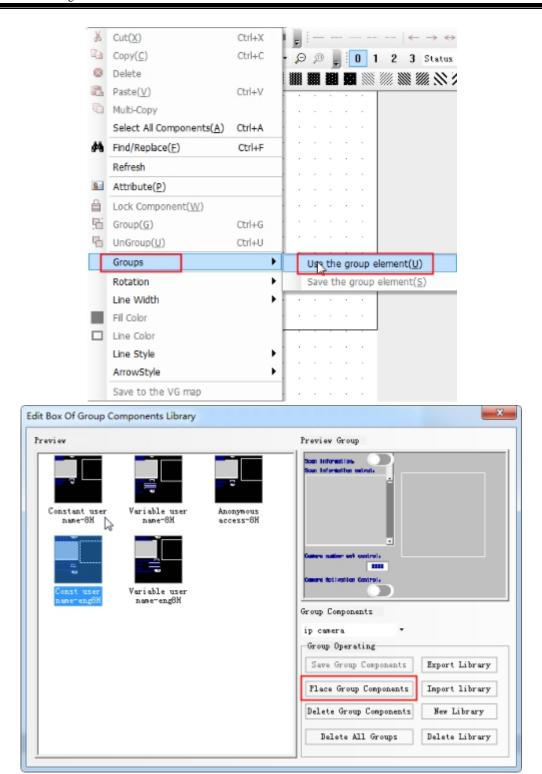
After placing the components, you can see that all components exist as a combined component. If you need to change the address of one of the components, you need to cancel the combination before you can change a single component.
