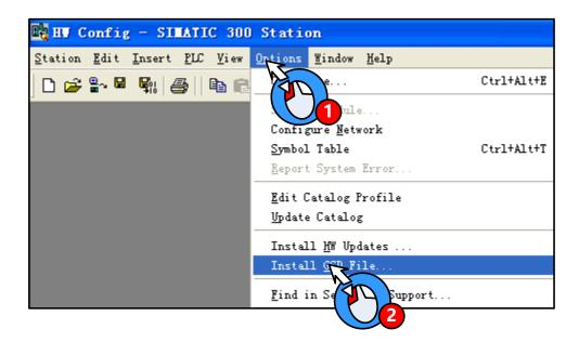
GSD file installed, Right in the HW Config directory PROFIBUS DP / Additional Field Devices / MMI find the appropriate configuration file:
