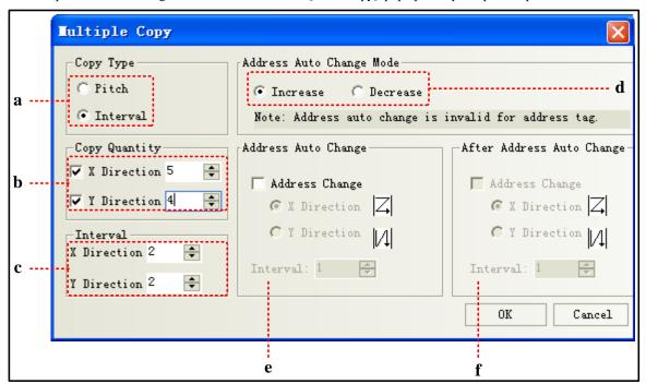
a: Interval makes the right border of the component as the start point to perform the copy. Pitch makes the 1<sup>st</sup> point in the upper-left corner of the component as the start point to perform the copy.
