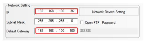
3) Assumed that the WAN IP of the local network where the HMI located is 203.110.174.214, then, users need to input 203.110.174.214:5900 and 203.110.174.214:5901 into PCs and mobiles of external network to remote control HMI.
