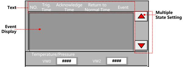
Ocreate new project [Event], and then add two windows Frame10 and Frame11 which are used for temperature alarm and pressure alarm. Set the attributes as follows:
