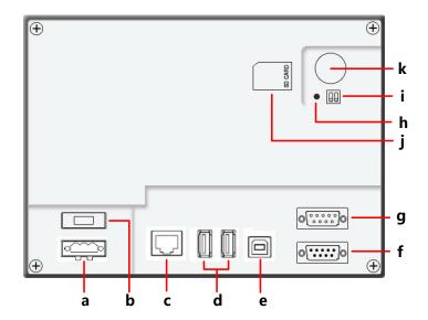
a. Input terminal of power supply DC24V b. 1A Fuse c. LAN interface d. USB HOST(USB type A interface) e. USB SLAVE(USB type B interface) f. COM1(male) g. COM0&COM2(male) h. RESET Button i. DIP Switch j. SD CARD interface k. One-time button type lithium battery
