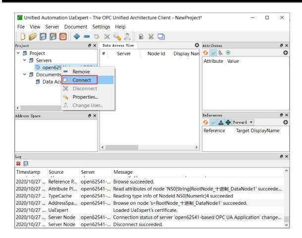
3) After the client is online with the HMI, it can automatically read the data nodes in the HMI, and can operate read or write the data nodes according to the set read-write attributes
