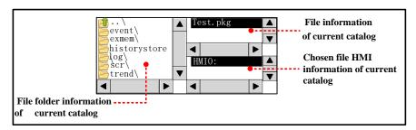
File list component is a special component; it is usually used together with the Import/Export function of Function Key.
