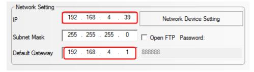
3) Assumed that the WAN IP of the local network where the HMI located is 192.168.100.14, then, users need to input IP 192.168.100.14 into VNC Viewer and mobiles of external network to remote control HMI. Choose menu "Network->WAN"
