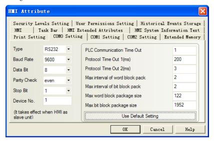
Them from the device number for the HMI station number, other communications parameters set according to specific circumstances.
