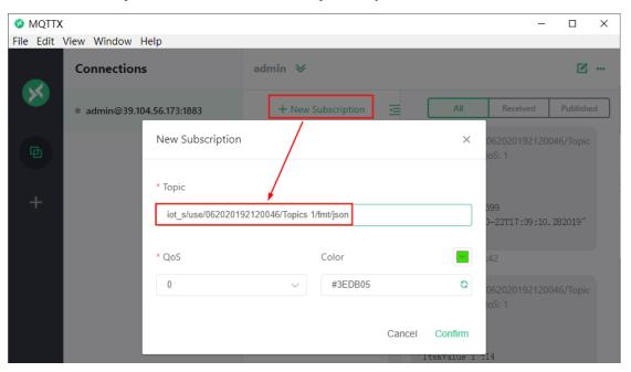
After adding, MQTTX software will receive data according to the cycle set in HMI; if you select cycle sending in HMI Software and check "send when data changes", then when HMI data changes, and wait for the set cycle, HMI will send the changed data.
