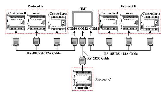
[Example] Below a GH070E with three MODBUS device (hereinafter referred to as PLC 0, PLC 1, PLC 2), a MITSUBISHI FX2N (hereinafter referred to as PLC 3), an OMRON CP1H (hereinafter referred to as PLC 4) communication is cases, Requirements were monitored on the HMI PLC 0, PLC 1, PLC 2 of 4X 100, PLC 3 of D100 data and PLC 4 of Q 0.0 outputs.
