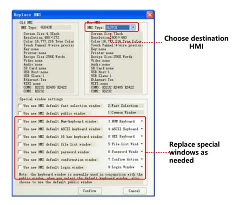
Choose the HMI you want in [] new HMI]- [HMI type], If resolution ratio of the two differ a lot, it is suggested to choose all the special windows, or the old ones are in use. Click OK to finish.
