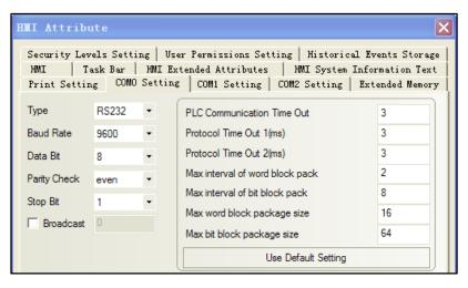
According to the actual physical connection mode selection set [Communication type].
