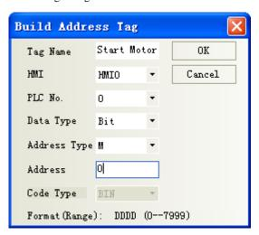
For example, build an address tag named "Start Motor", the address is M0. Click on the OK to finish building this address tag, and click on Cancel to give up this address tag.
