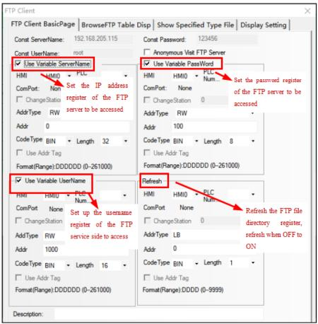
The effect of accessing the HMI FTP files is as follows
