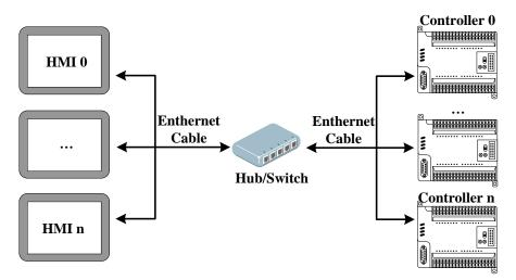
[Examples] Below two GH070E (hereinafter referred HMI0 and HMI1) and one MODBUS TCP device (hereinafter referred to PLC0), and one OMRON CJ series PLC (hereinafter referred to PLC1) communications as an example. Require to monitor the data of PLC0 4x100 in the HMI0, and to monitor the data of PLC1 D100 in HMI1.
