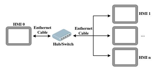
[Example] Below two GH070E communication, for example, requires HMI0 screen control HMI1 of LB100 status output to ON.
