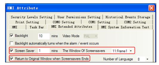
When the HMI screen in the set period of time without touched, the screen will switch to the specified window that screensaver window.
