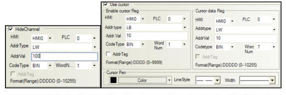
Set LW. B100.0 to ON, Channel 0 will be hidden; Set LW. B100.1 to ON, channel 1 will be hidden and so on.
