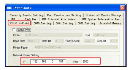
**4** In the [HMI Attribute]-[HMI], set the HMI IP address
